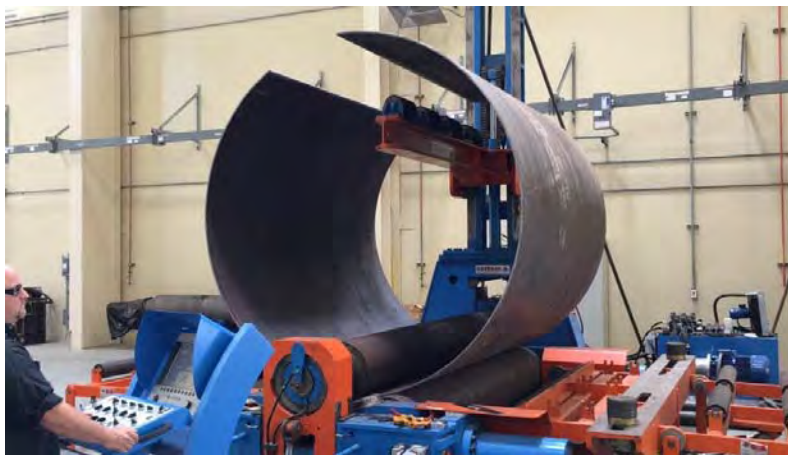
Pipe being rolled at Metropolitan’s La Verne Shops
