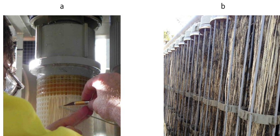
Figure 1 - a) Cutting a single fiber from a drinking water membrane and b) membrane modules that have been recently removed from an MBR.
