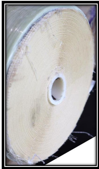
Figure 16: No telescoping was observed on the concentrate end of the element.
