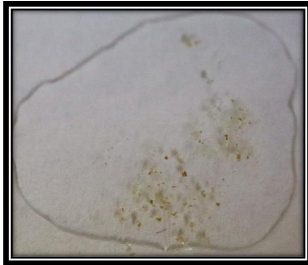
Figure 27: No effervescence was observed upon the addition of acid to the dehydrated foulant.
