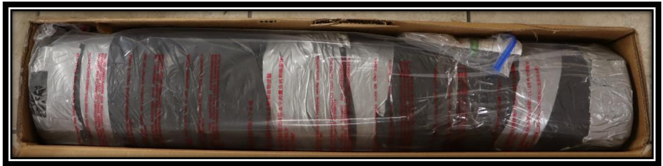
Figure 4: The element was placed inside membrane bags and closed with tape.
