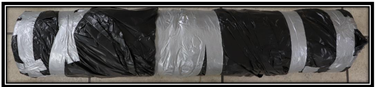
Figure 5: The element was placed inside plastic bags and closed with tape.
