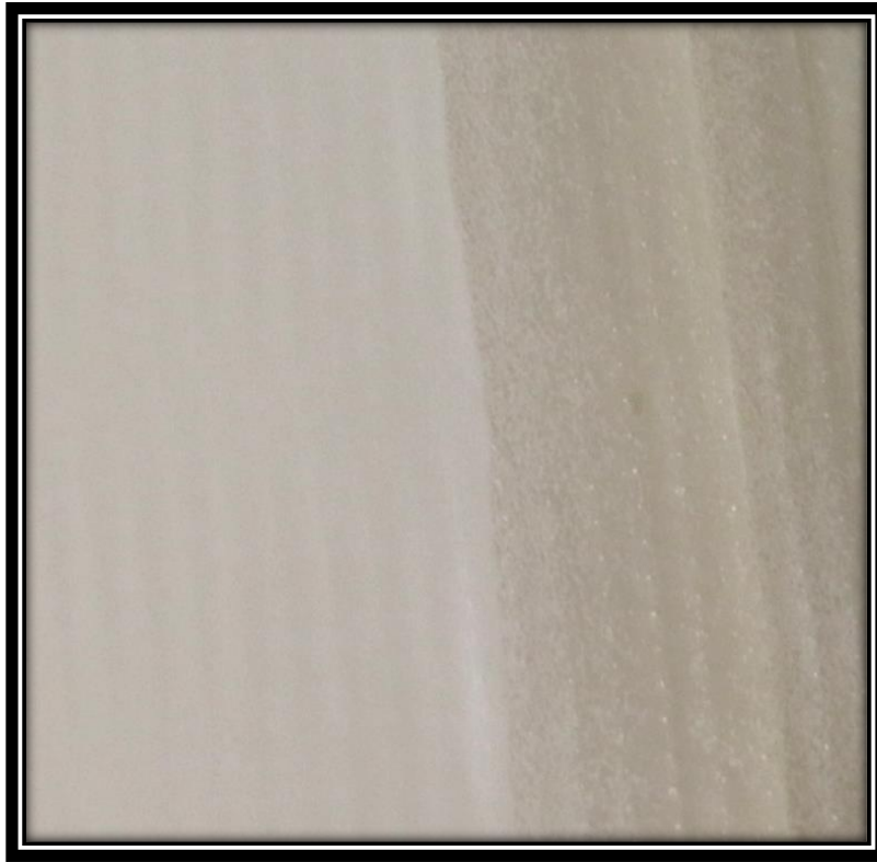
Figure 22: No osmotic bubbling was observed along the glue line.
