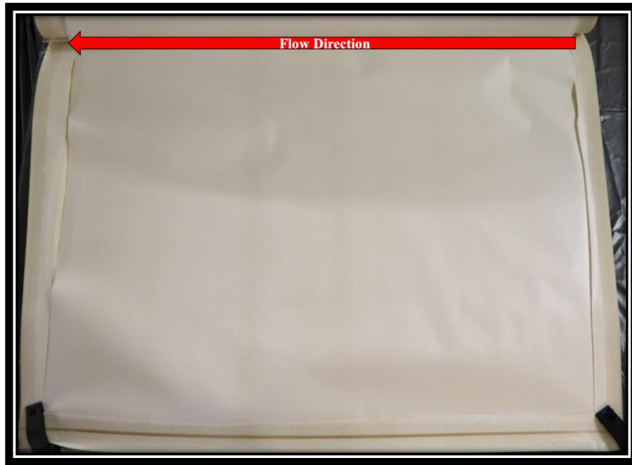
Figure 23: The permeate side of the membrane.
