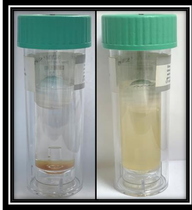
Figure 45: SLYM – start (left), negative for slime forming bacteria (right).
