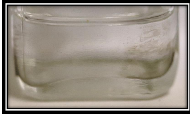
Figure 26: The dehydrated foulant was not visibly soluble in the ~37% HCl solution.
