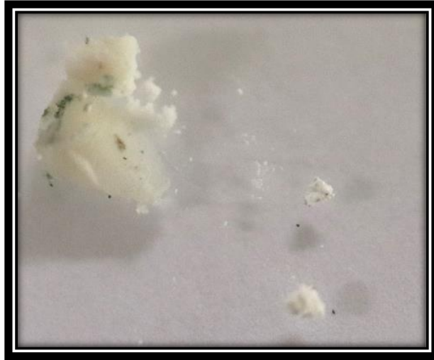
Figure 47: White material from pressure vessels sample arrived with the membrane.
