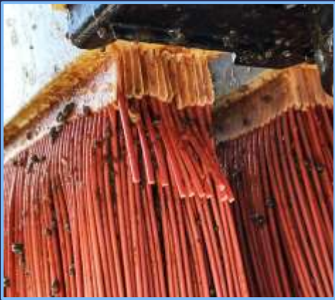
Membrane element closeup during challenge testing
