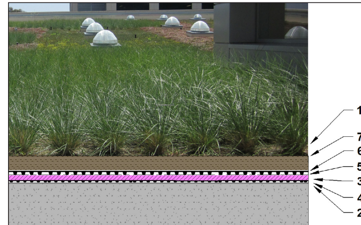
Typical components of an extensive green roof. The cross section of intensive green roofs will be deeper and vary from site to site based on desired functions and structural capacity of the underlying structure.
