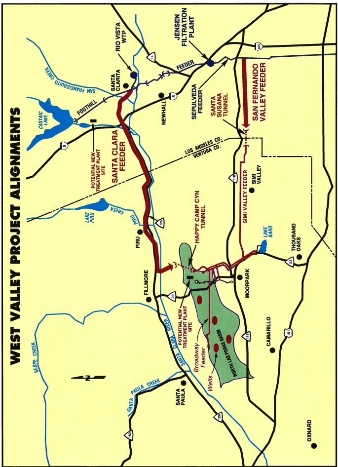
alignments would probably be in the same general vicinity of faults as the existing West Valley Feeders and Santa Susana Tunnel. Should a slip along a fault in the vicinity of the existing West Valley Feeders occur, the existing feeders as well as a new San Fernando Feeder may be subject to the same impact because of the pipelines' proximity to each other.
