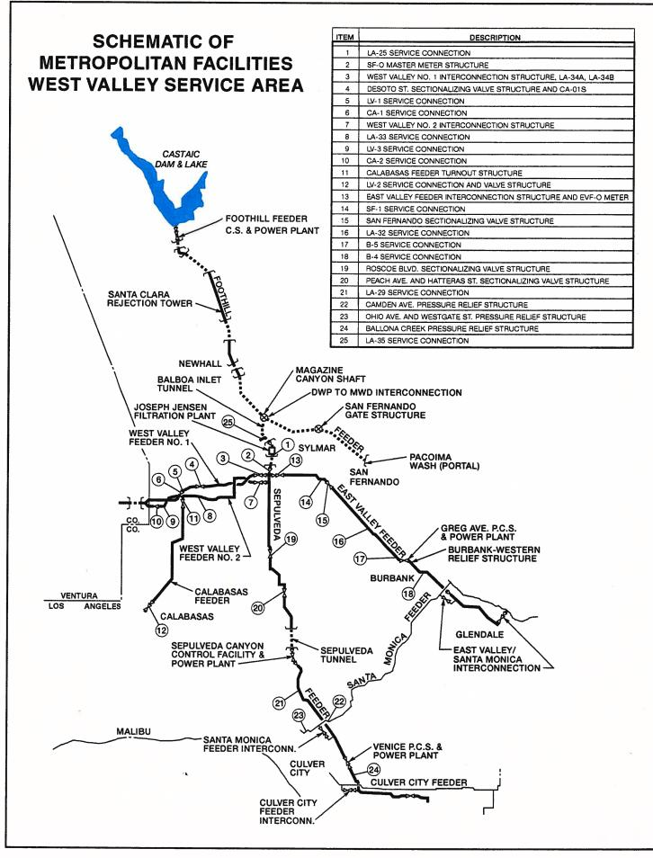
released through the proposed LA-36 service connection into Pacoima Wash or continue southerly through the Balboa tunnel to the Jensen plant. LADWP can also take delivery of state project water through LA-35 which is located just upstream of the Jensen plant. These deliveries are treated by LADWP along with its own imported supplies through the LA Aqueduct Filtration Plant.
