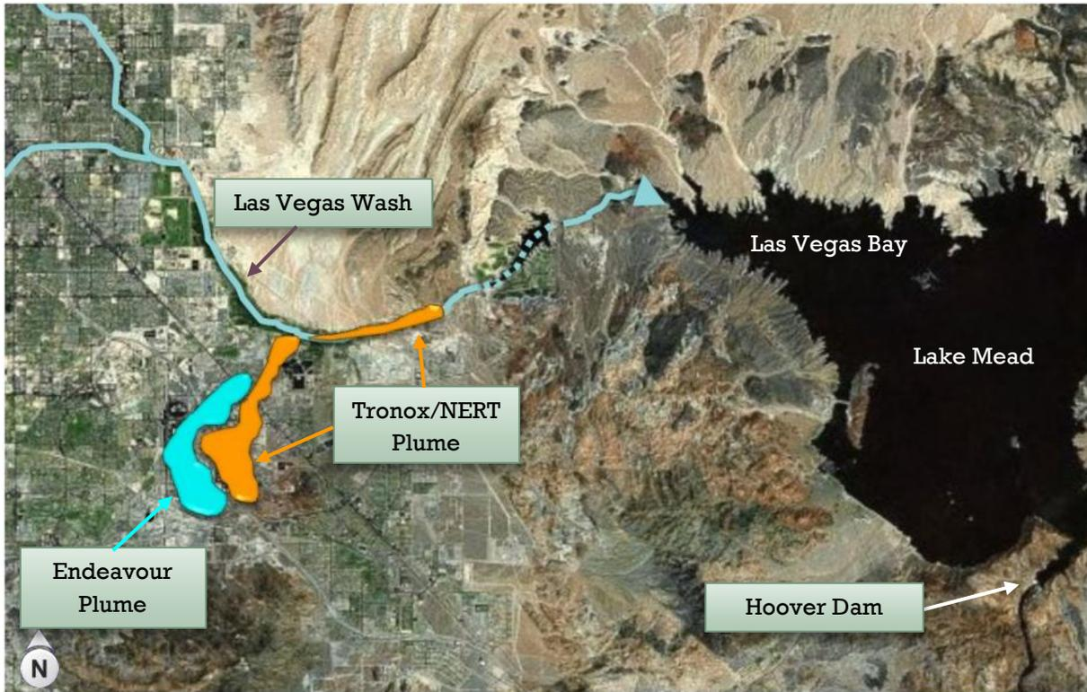
Figure 6-12. Tronox and Endeavour Perchlorate Plumes
