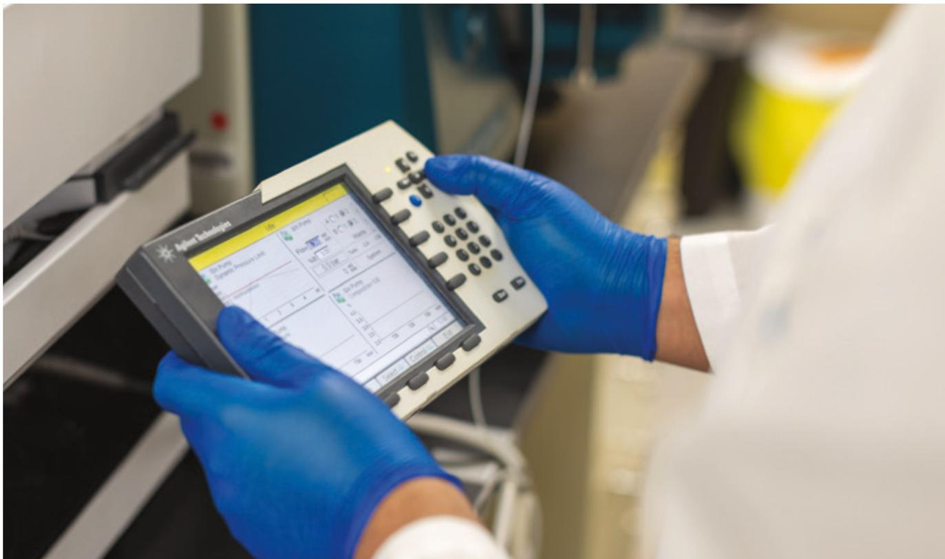
» Instrument control module for water quality analysis.
