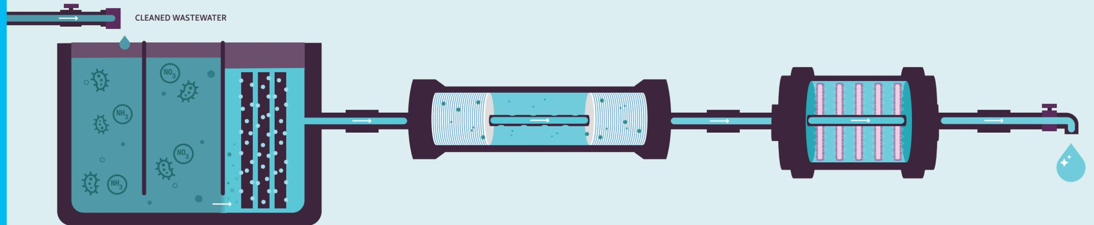
**1 Membrane Bioreactors:** Microorganisms remove ammonia and other nitrogen compounds, while membranes filter tiny particles, including microorganisms smaller than 1/100 of a grain of sand.
