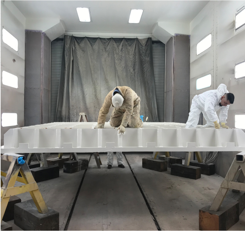
Staff coating a bypass slide gate and frame for the Skinner Water Treatment Plant.
