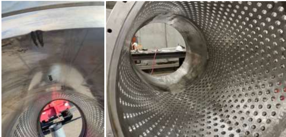
Damage discovered on outer valve body (left) and completed weld repairs (right) for Red Mountain PCS
