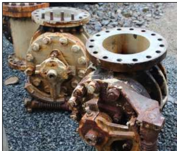
Corroded valves removed from the Santiago Lateral
