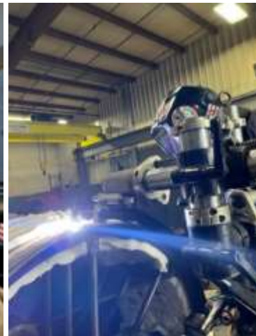
Vendor performing machining work (left) and overlaying hard-face material on valve gate (right) for Red Mountain PCS
