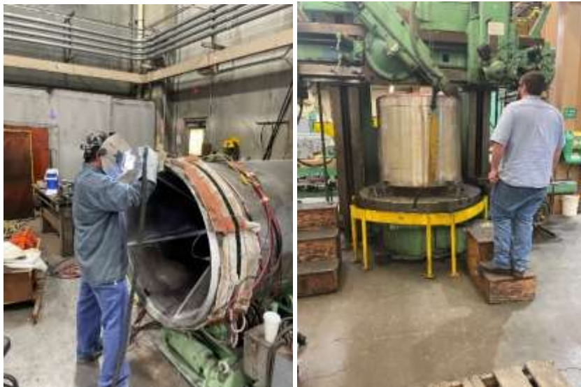
Staff weld-repairing valve gate (left) and machining of inner valve body (right) for Red Mountain PCS
