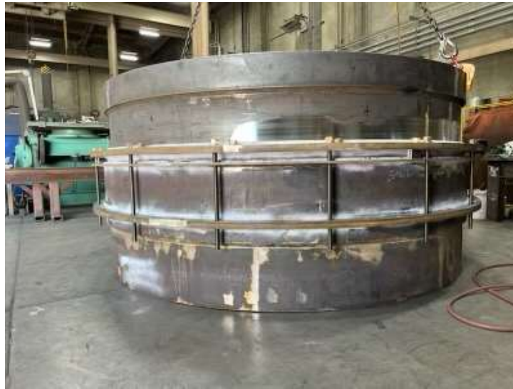
Fit testing of the manufactured slip joint for repairs on the Upper Feeder
