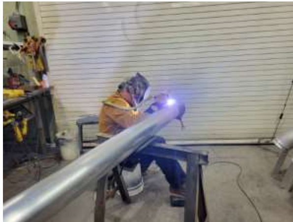
Staff fabricating a pipeline for a portable pump to dewater during the CRA shutdown
