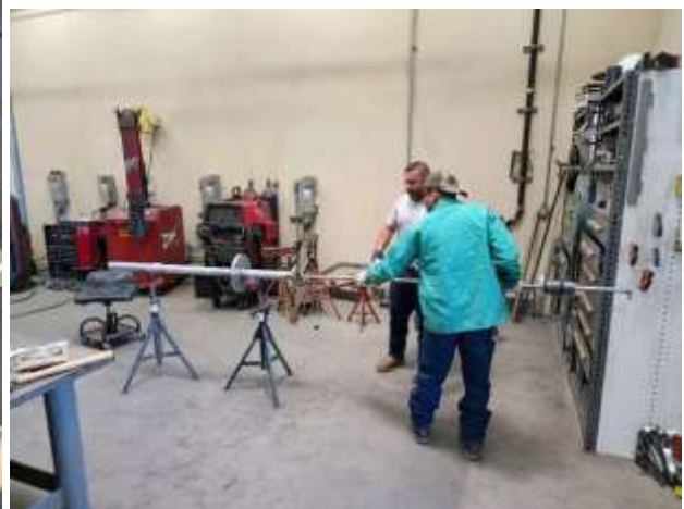
Double containment piping (left) and new containment lance (right) for fluoride injection feed line at the Weymouth plant
