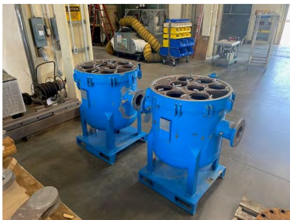
As-received set of quagga filters received (left) and prepping for abrasive blast of filters (right)
