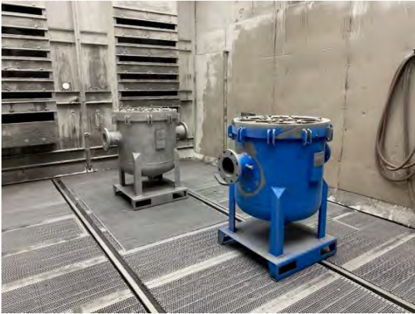
Abrasive blast in process (left) and post blast assessment (right)
