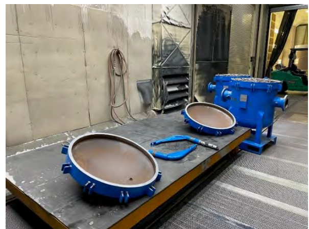
As-received set of quagga filters received (left) and prepping for abrasive blast of filters (right)
