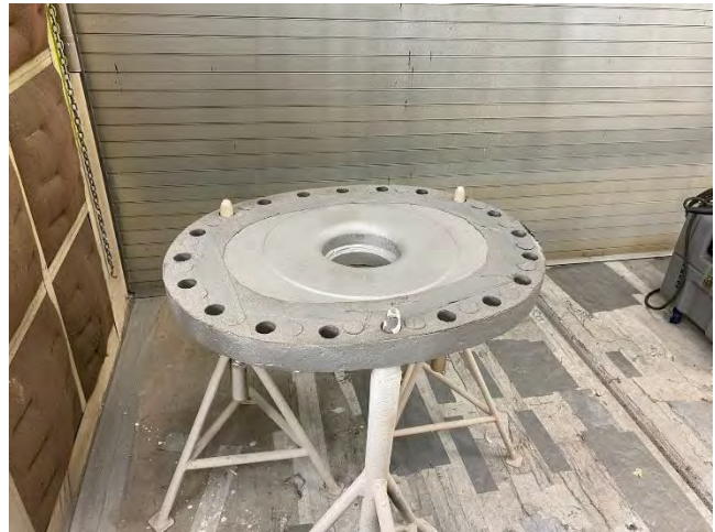
Welding completed on elliptical flange (left) and completed abrasive blasting (right)
