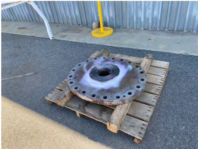
Welding completed on elliptical flange (left) and completed abrasive blasting (right)
