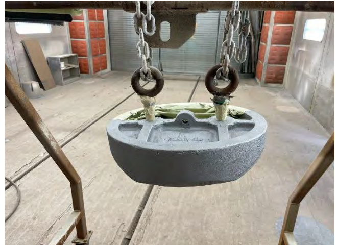
As-received boiler plate and elliptical flange (left) and boiler plate in blasting process (right)
