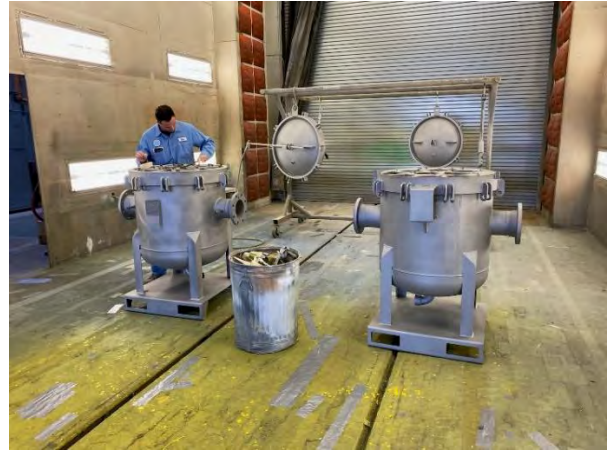
Abrasive blast in process (left) and post blast assessment (right)
