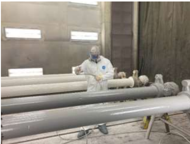
Applying finished coating to the stems (left) and delivery of completed stems (right) for DWR's San Luis Dam Head Gate
