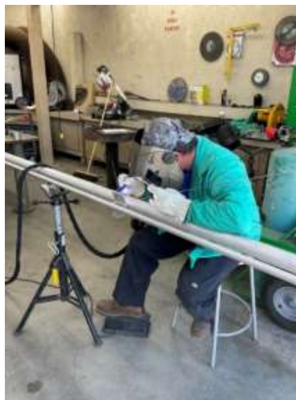
Staff constructing a new caustic soda diffuser at the Skinner plant
