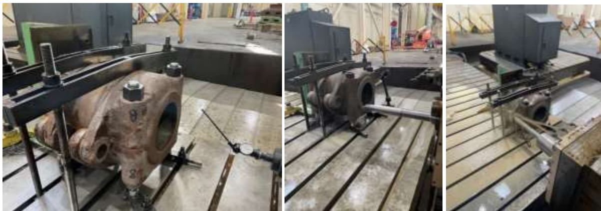
Fixturing of coupling assembly (left) and line boring of coupling hinge (center and right) for DWR's San Luis Dam Head Gate
