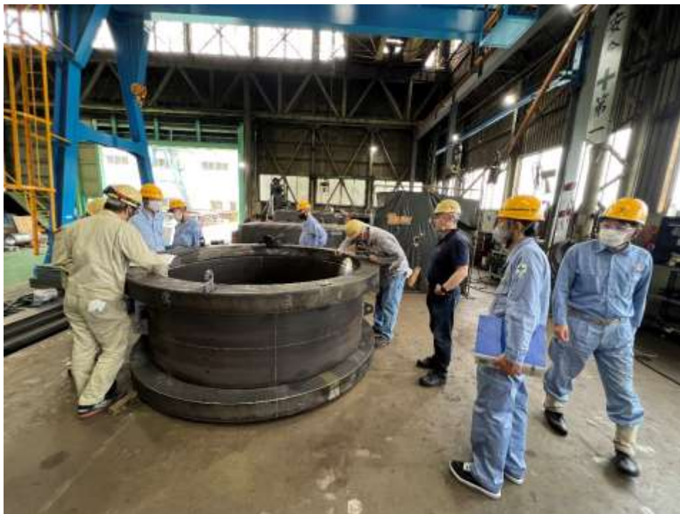
Badlands Tunnel Surge Tank Project —Valve inspection by Metropolitan staff and contractor personnel
