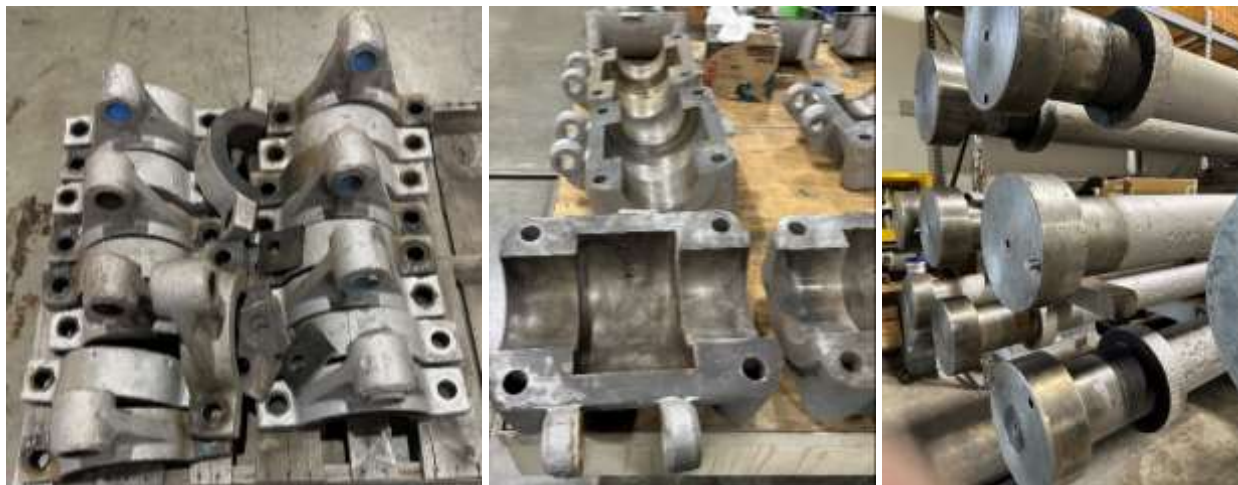
Post abrasive blast condition of clamps (left), couplings (center), and stems (right) for DWR's San Luis Dam Head Gate
