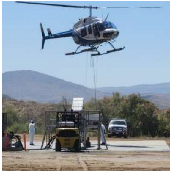
Staff refilling the helicopter's hopper with granular copper sulfate for application at Lake Skinner
