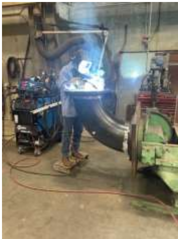
Survey report of the existing elbow (left), fabrication of new elbow (middle), and installed new elbow (right) at the Weymouth plant
