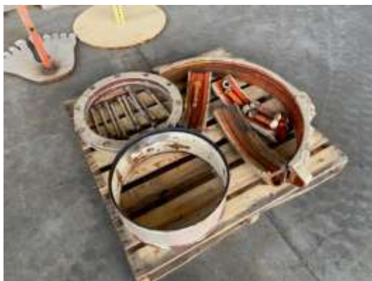
Victaulic and Dresser couplings before (left) and after refurbishment (right) for the Weymouth plant
