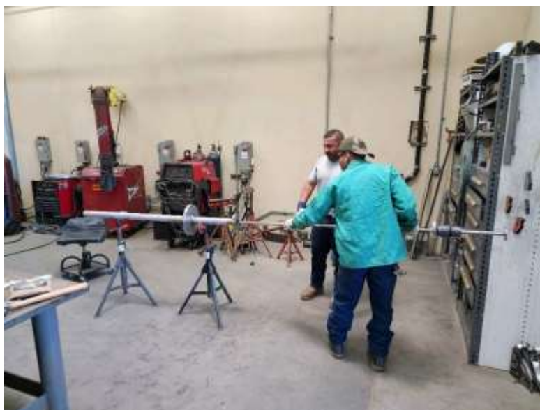
Staff fabricating new injection lance for the fluoride system at the Weymouth plant
