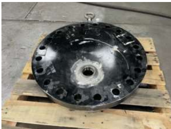
Fabricated 30-inch blind flange before (left) and after (right) coating application for the Second Lower Feeder shutdown
