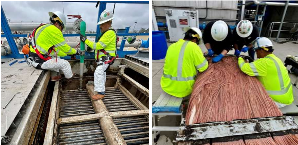
Staff removing a membrane cassette (left) and cutting membrane fibers (right) for compromised membrane testing at the demonstration plant
