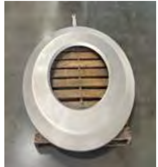
Engineering drawing (left) and completed orifice plate (right) for service connection USG-03
