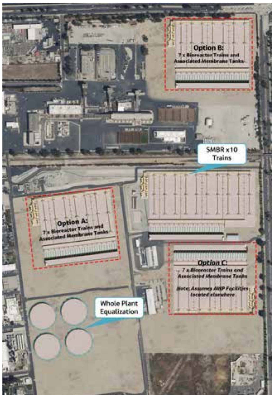
Figure 7-10. Whole-Plant Flex MBR – Secondary Operation
