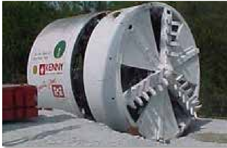
Figure 3-7 Open Mode Shielded TBM used on Cady Marsh Stormwater Tunnel, Griffith, Indiana
