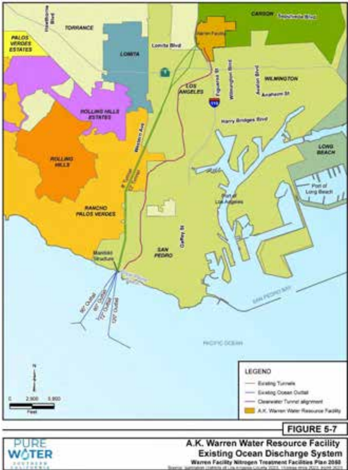
Figure 5-7. A.K. Warren Water Resource Facility Existing Ocean Discharge System
