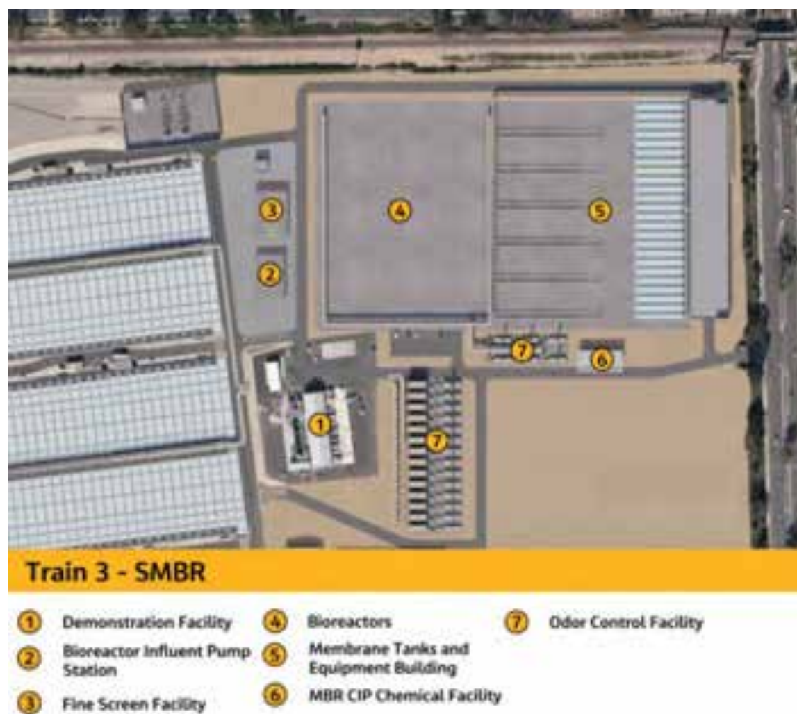
Figure 6-2. Greenfield SMBR Site Plan General Layout
