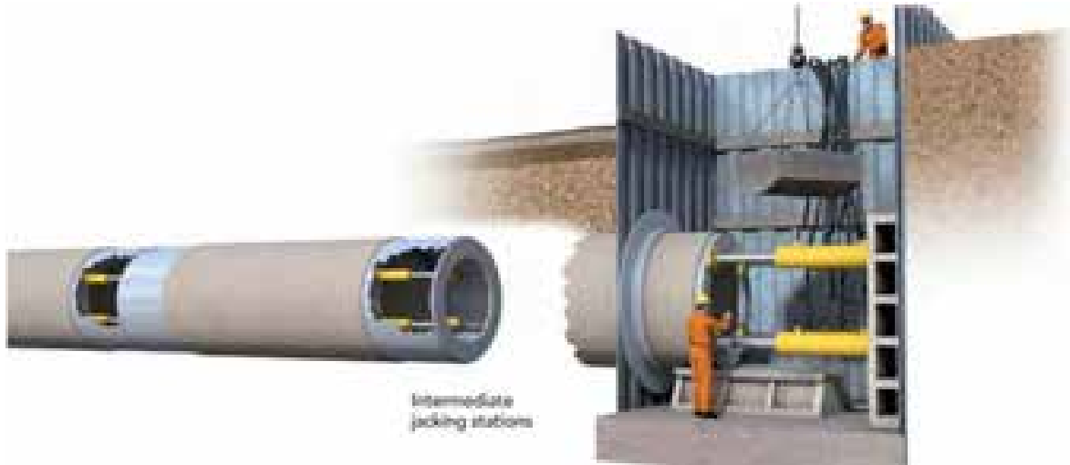
Figure 3-5 Interjack Stations and Jacking Portal, Pipe Jacking Association
