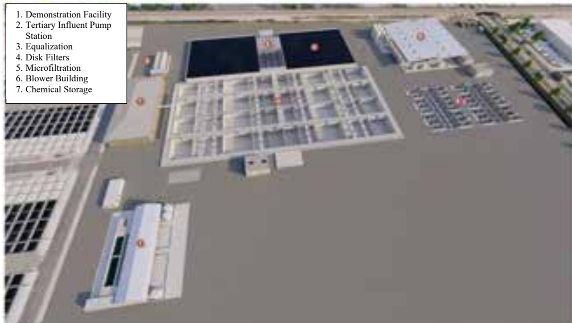
Figure 6-4. TMBBR Site Plan General Layout
