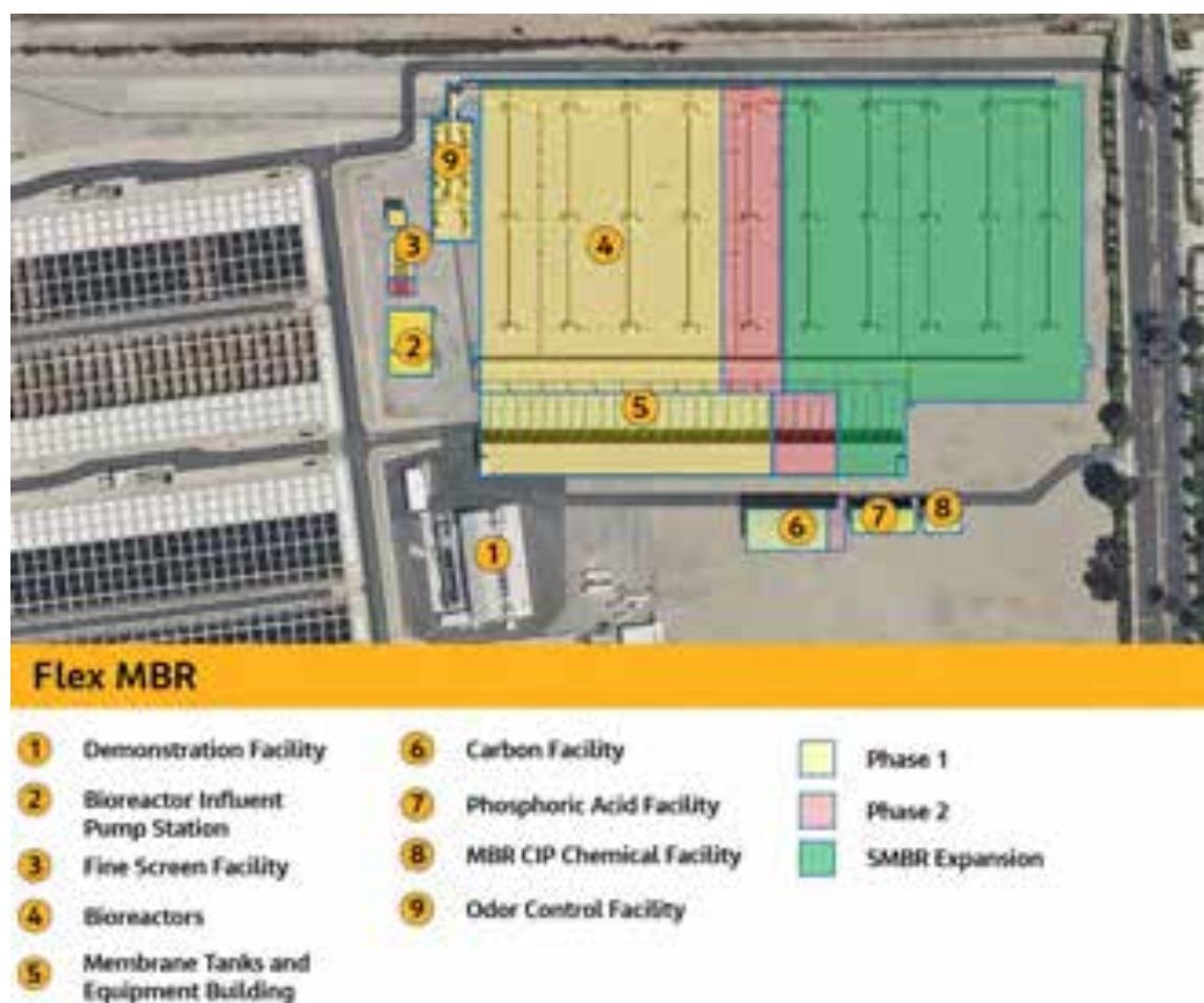
Figure 7-6. Flex MBR Site Plan Phasing to 150-MGD Secondary Operation
