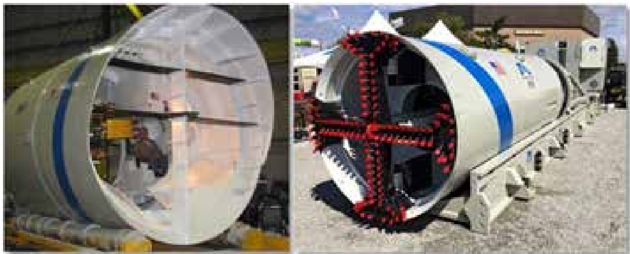
Figure 3-3 Boring/Digger Shield and Cutting Head, Akkerman
