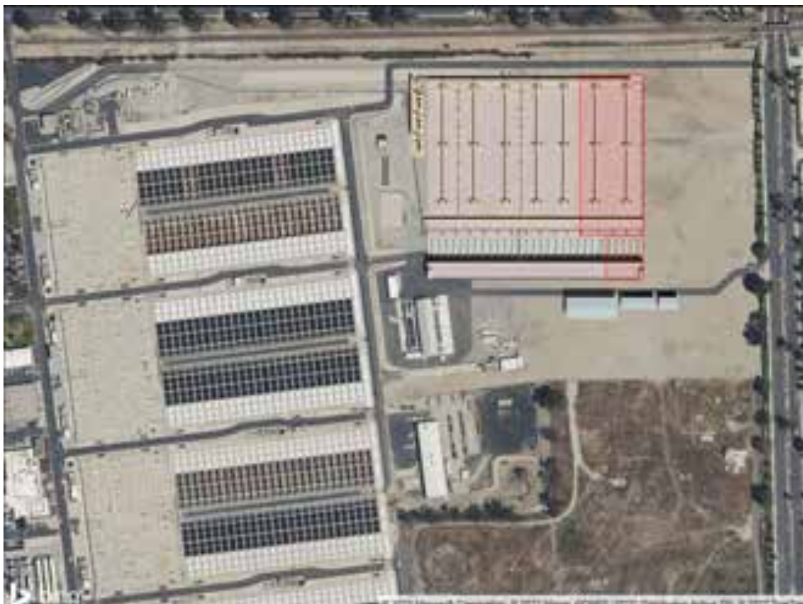
Figure 7-8. Expanded Reuse (180 MGD Produced Flow) Train 1 (Flex MBR - Tertiary) Conceptual Site Plan
