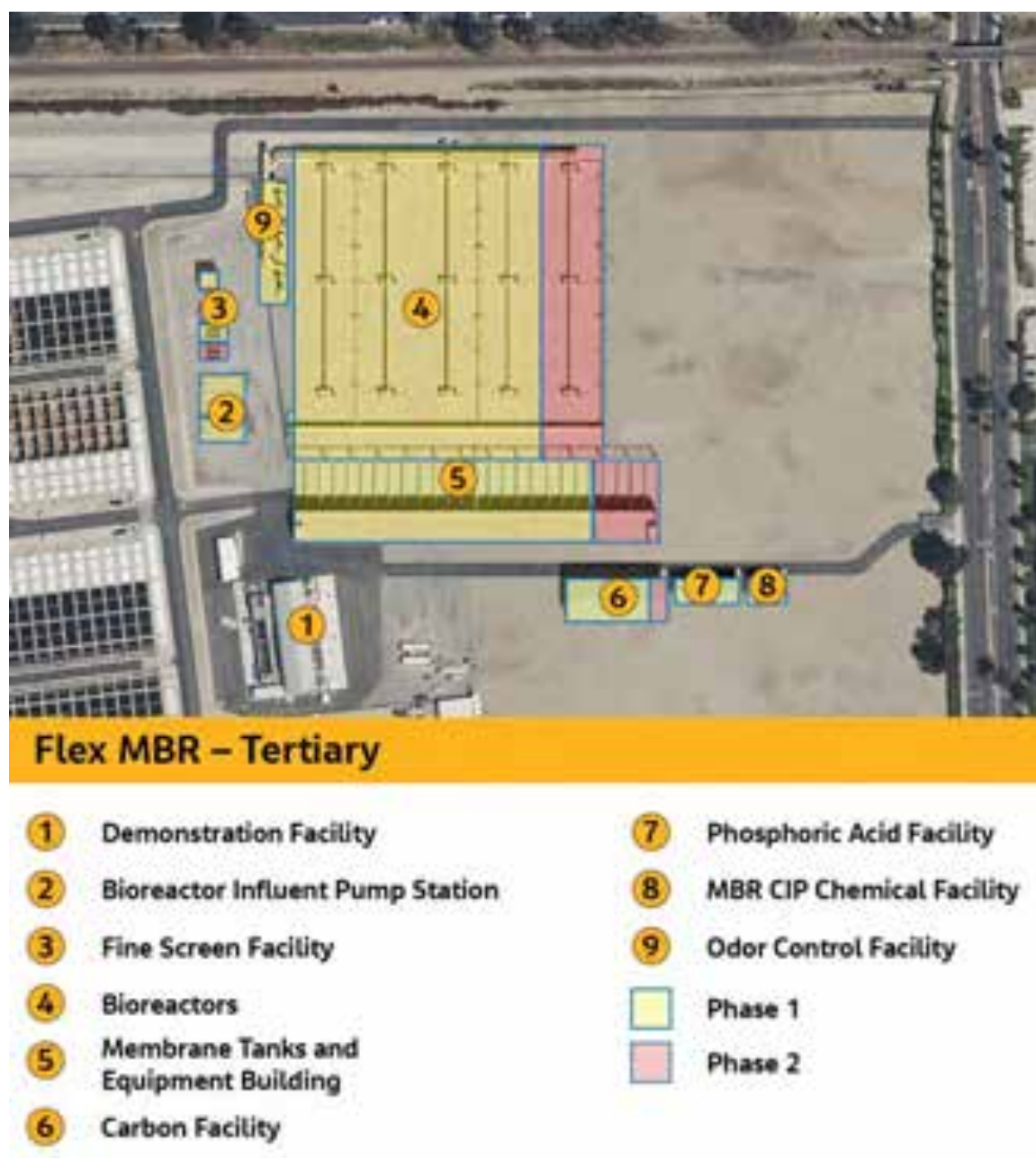
Figure 7-4. Flex MBR Site Plan Phasing to 150-MGD of Tertiary Operation
