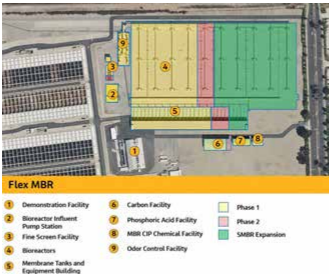
Figure 6-3. Flex MBR Site Plan General Layout
