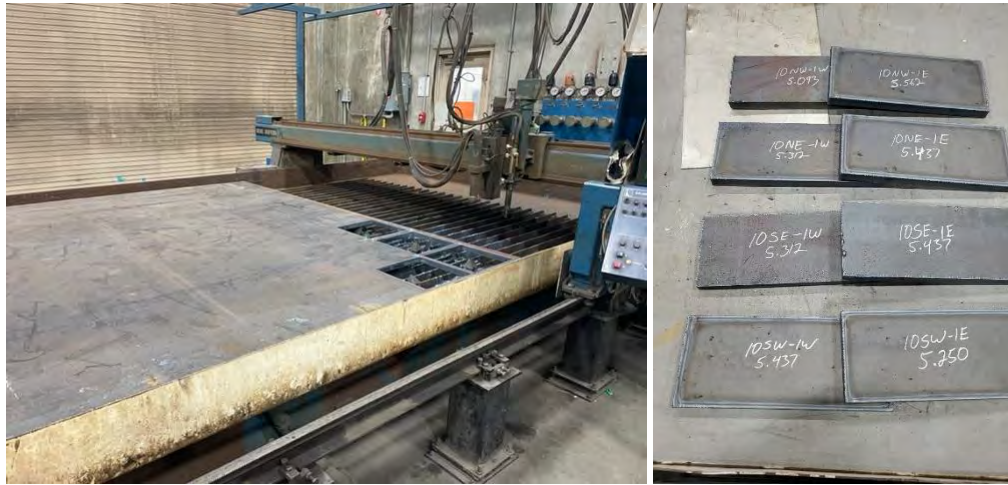
Cutting carbon steel plate (left) and four sets of cut plates (right) for Basin 10 at the Jensen plant
