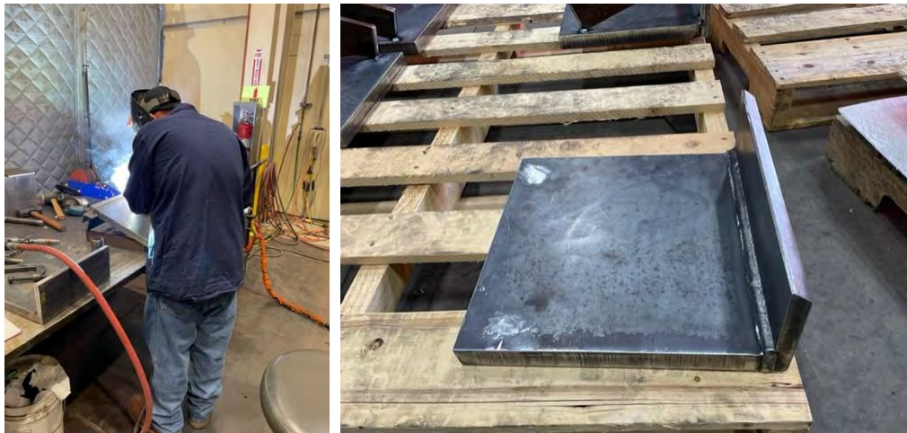
Staff welding custom flocculator base plate (left) and completed base plate (right) for repairs at the Jensen plant
