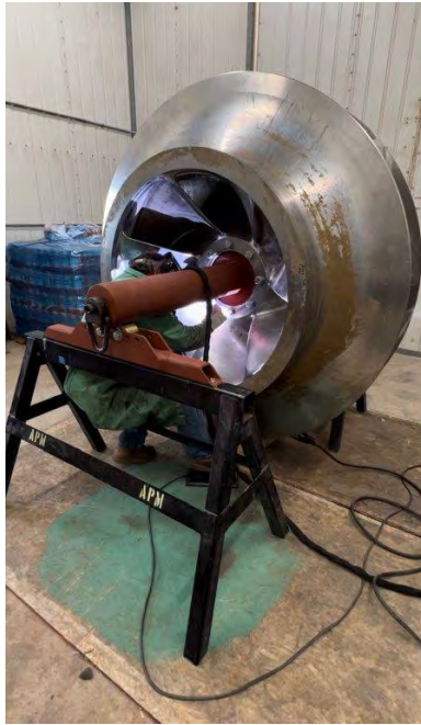
Staff repairing a pump unit impeller at Iron Mountain pumping plant
