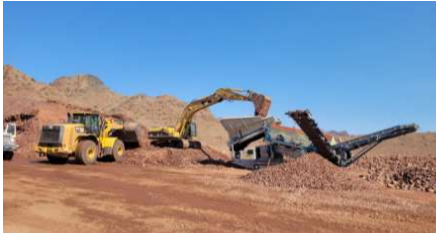
Staff processing base material through a screening machine for separation into various size aggregate at a Desert facility
