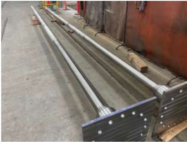
Completed manufacturing of center post (left) and machining of the gate's lower bearing (right) for DWR
