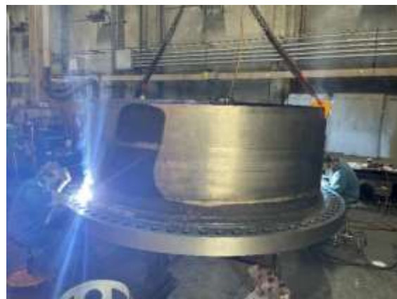
Staff welding flanges to upstream thimble (left) and downstream thimble (right) for the Upper Feeder repairs
