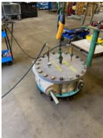
Pressure testing of the refurbished valve (left) and completed valve (right) ready for transport to the Perris Pumpback facility
